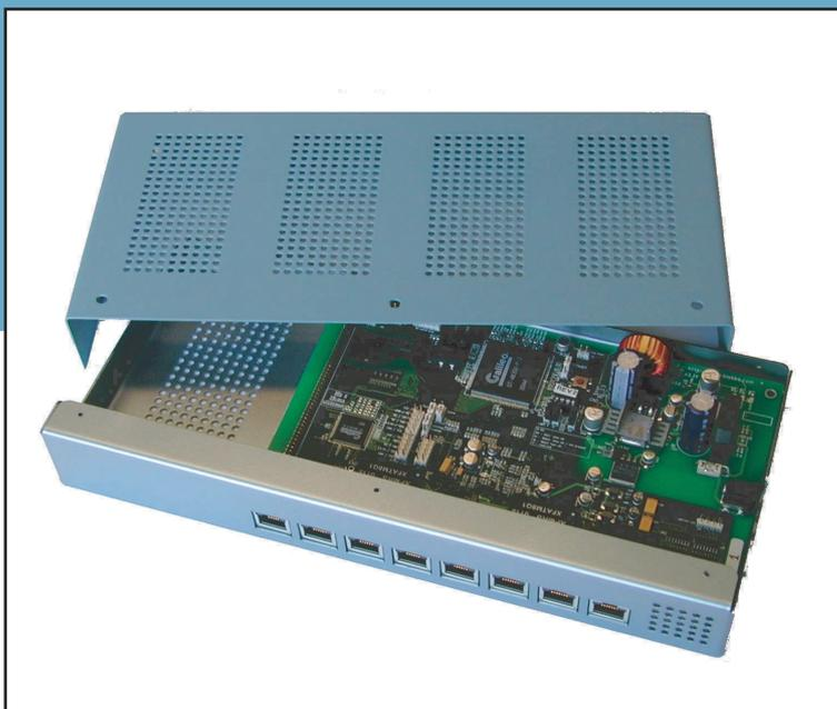
Without Quality of Service a video-on-demand film could be interrupted if someone else in the family started using other broadband services and home appliances. To ensure QoS, the multimedia switch has prioritized ports for different kinds of services and it has the necessary Layer Three software to handle IGMP-snooping for Quality of Service in multicasting.
